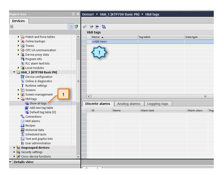
In the project tree, navigate to HMI\_1, expand and double-click "Show all tags" under the 'HMI tags' folder.
