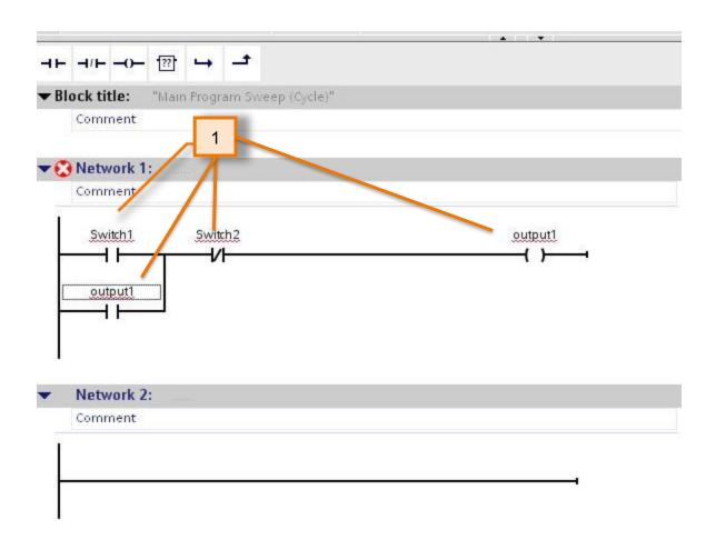
1. Type in the symbol names as shown: Switch1, Switch2, and Output1 (for both coil and "seal").
