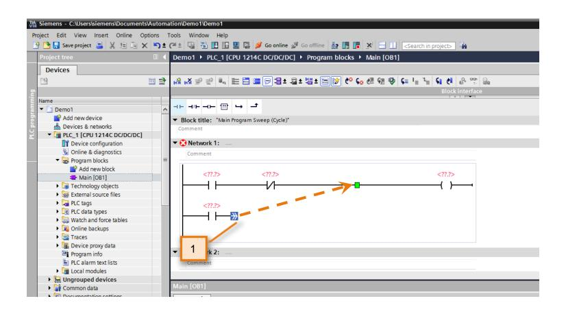
Drag the connection from the contact to the position as shown.
