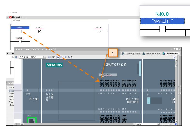
Drag and drop the text 'Switch1' directly on top of input address 'I0.0' on the PLC hardware.
