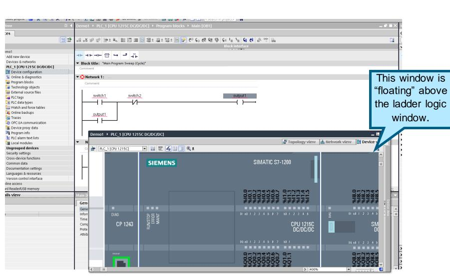
Make sure that the zoomed in PLC hardware window floats above the ladder logic window as shown. You might have to resize the floating window.
